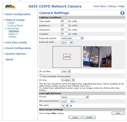
To compensate for the lighting conditions, the Color level, the Brightness, the Sharpness, the Contrast, and the exposure control, the exposure area and the IR cut filter can all be adjusted. DC-Iris should always be enabled, except when focusing, or when using a non-DC-Iris lens.
